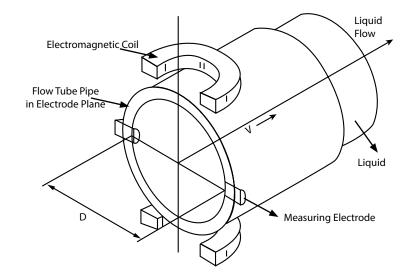
The induced voltage is not affected by the physical properties of the liquid like temperature, viscosity, pressure, density and conductivity, as long as the conductivity of the measured liquid is above a minimum threshold.
