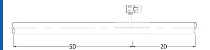
At flowmeter upst ream, there should be straight pipe no less than 5D and no less than 2D at flowmeter downstream. (D is the inner diameter of flowmeter)
