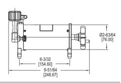
The Model LPCP Low Pressure Calibration Pump is a low air pressure source with the ability to easily adjust and stabilize. It is made up of quick connectors for fast instrument connect and disconnect.
