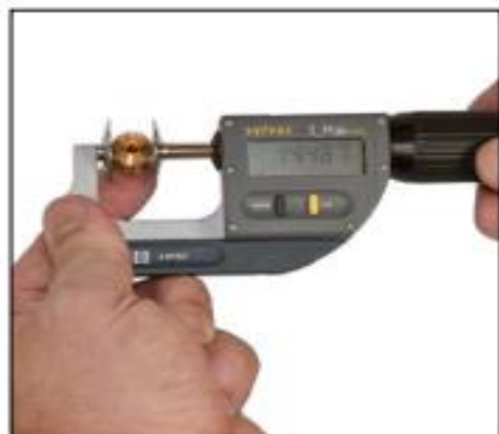
Part measurement with a S_Mike PRO Disk
