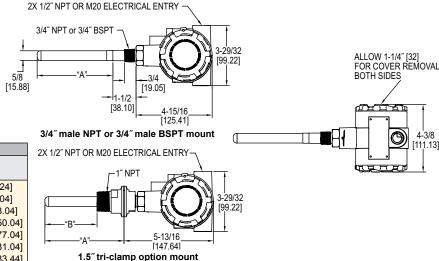
Service: Air and compatible gases, any type of particulate conductive or non-
