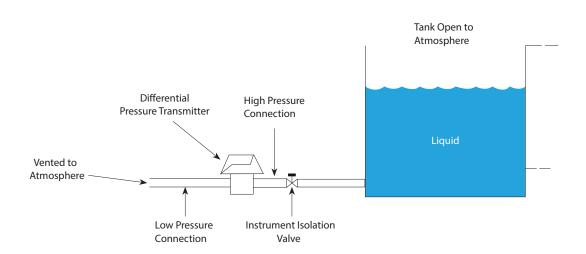
The above mentioned equation shows that the liquid level is directly proportional to the hydrostatic pressure. Therefore, as the liquid level increases, the hydrostatic pressure measured at the high-pressure port also increases.
