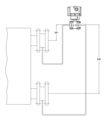
Installation of transmitter between the measuring points, no vaccum
