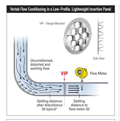
Model VIP flow conditioners marry the scientifically proven superior performance of Vortab tab-type flow conditioning technology with the installation ease and cost savings of an insertion panel design.
