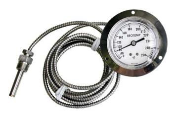
Note: Thermowells should be used whenever the stem or bulb would be exposed to pressure, corrosion, velocity, abrasion or shear forces. Thermowells also make it possible to remove the thermometer without losing pressure or the contents of the process.
